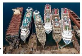
and try to milk every last bit of value out of it, from the steel in the superstructure that is used to make rebar for construction projects around the world to things like artwork, decking and even toilets.
