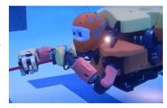
items picked up by the unit. It also offers eight multidirectional thrusters and stereoscopic vision that allow it to be operated in sensitive environments.
